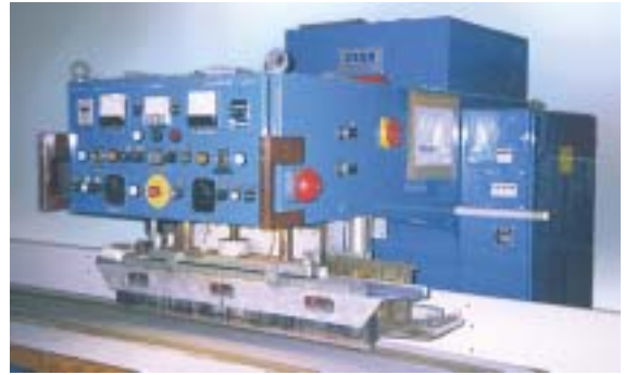
High Frequency Welding Machine for Flex pvc T-GRIP™
