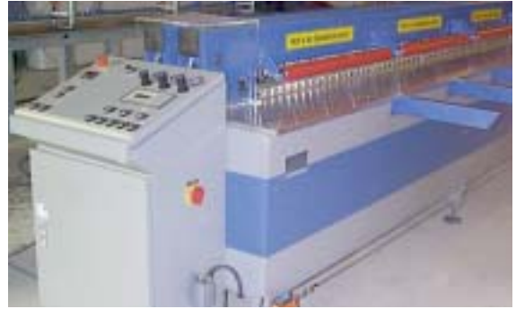
Butt Welding Machine for HDPE T-GRIP™
